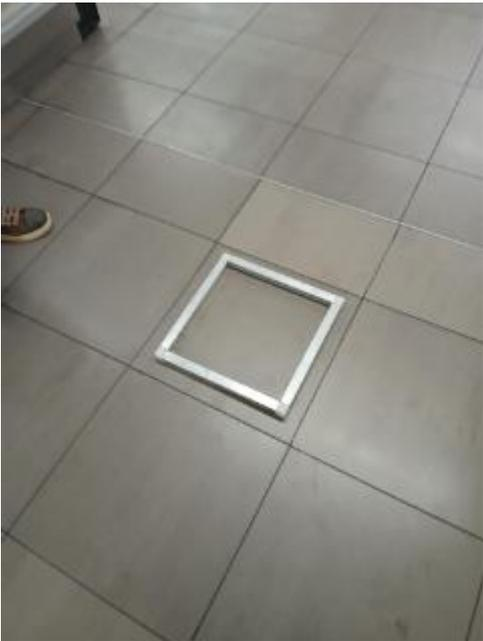
A photograph showing a square, silver-colored metal sampling frame placed on a light-colored tiled floor. The tiles are square and laid in a grid pattern. A person's foot wearing a brown shoe is partially visible in the upper left corner.  | <p>00629247-P01 - <b>12,4 <math>\mu\text{g}/\text{m}^2</math></b><br/>R-1 - Quai RER D<br/>Voies 1-3<br/>ESC HALL 2<br/>Au sol</p> <p>Revêtement : Carrelage</p>         |
