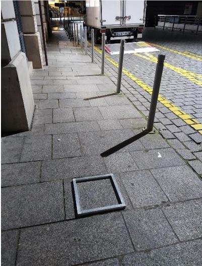
A photograph showing a public square area paved with granite slabs. A square metal frame is placed on the ground, indicating the sampling point. In the background, there are metal stanchions and a white truck. | <p>601193-P04 -279,6 <math>\mu\text{g}/\text{m}^2</math><br/>Parvis public<br/>Arrière hôtel<br/>Voir plan et photographies<br/>sur Sol<br/>Revêtement : Dalle granit</p>            |
